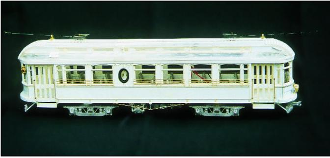
Before and after! The unpainted model (above) shows the interesting mix of materials that Bob Robbins employed to build Illinois Traction System car No. 203 in O scale. The predominant material is white Evergreen styrene, augmented with
