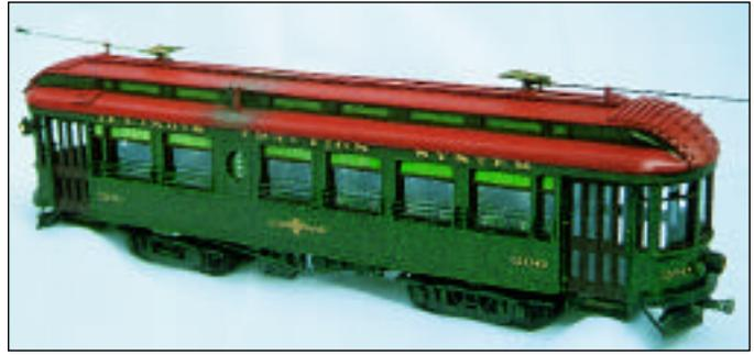
brass wire and detail parts and white-metal castings (including the truck sideframes). The roof is a clear styrene part manufactured by Vane Jones. Construction of car No. 200 is identical; the model was painted by Dennis Love.
